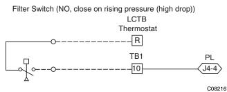
Fig. 54 - PremierLink Filter Switch Connection
